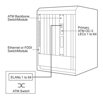
Figure 1-4 Example Base Configuration
